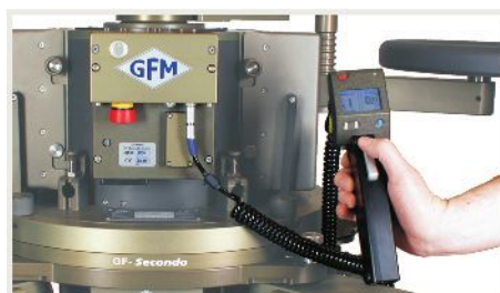
GF-Secondo with cable connected HCU
