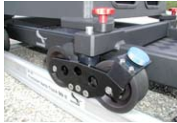
brake for track wheels
